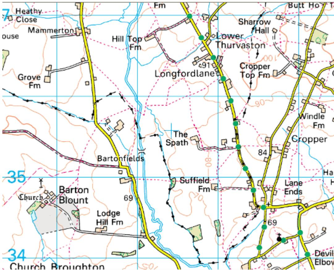
Figure 1 Sutton Brook. Note the mostly straight channel, compared with the natural meandering plan-form evident adjacent to Lodge Hill Farm.
