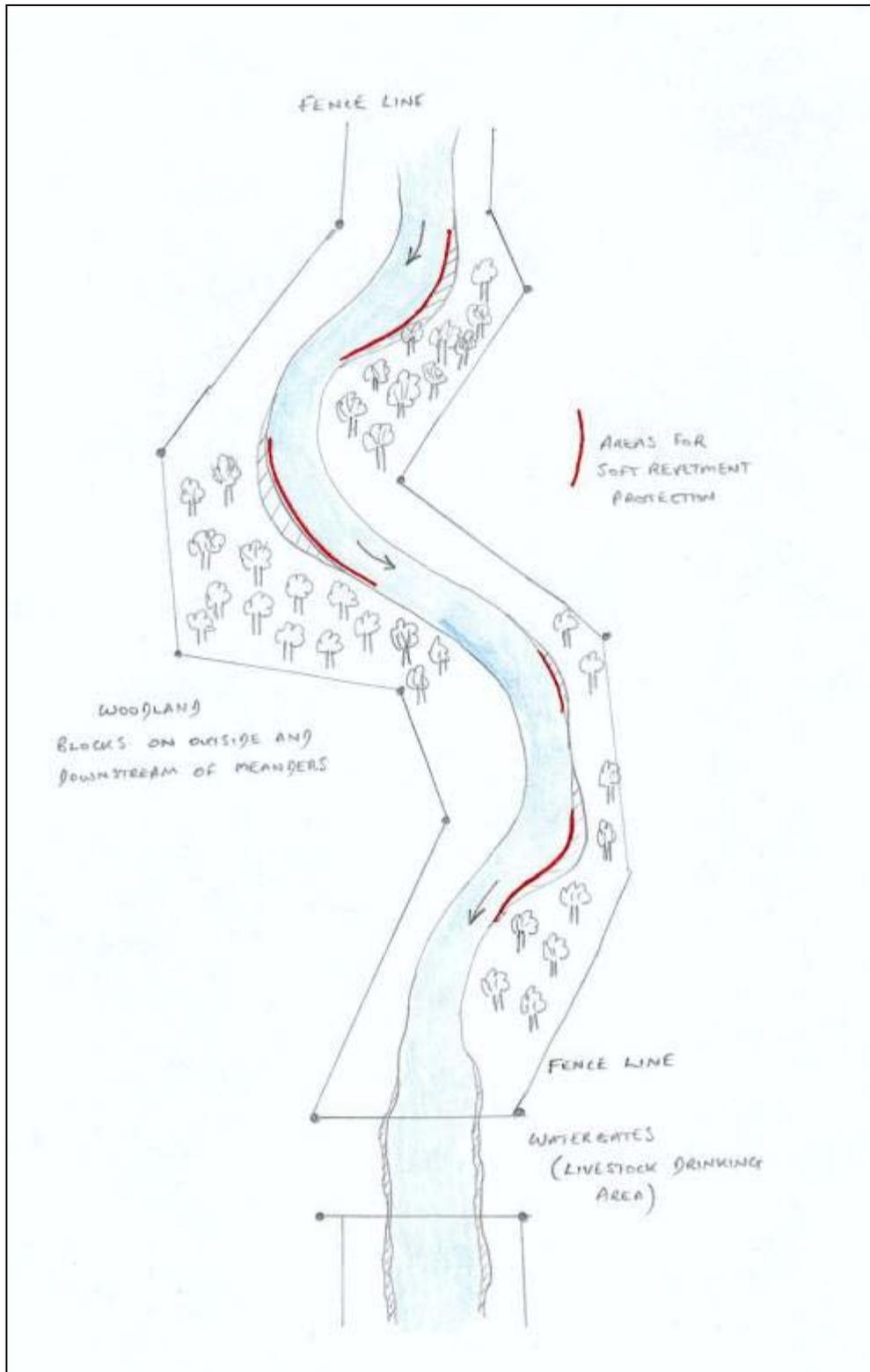
Figure 3 Creating buffer zones alongside the river and strategic tree planting, combined with soft revetment of currently eroding banks, could significantly increase bank stability and habitat quality. Fencing is only required if fields are used for livestock.
