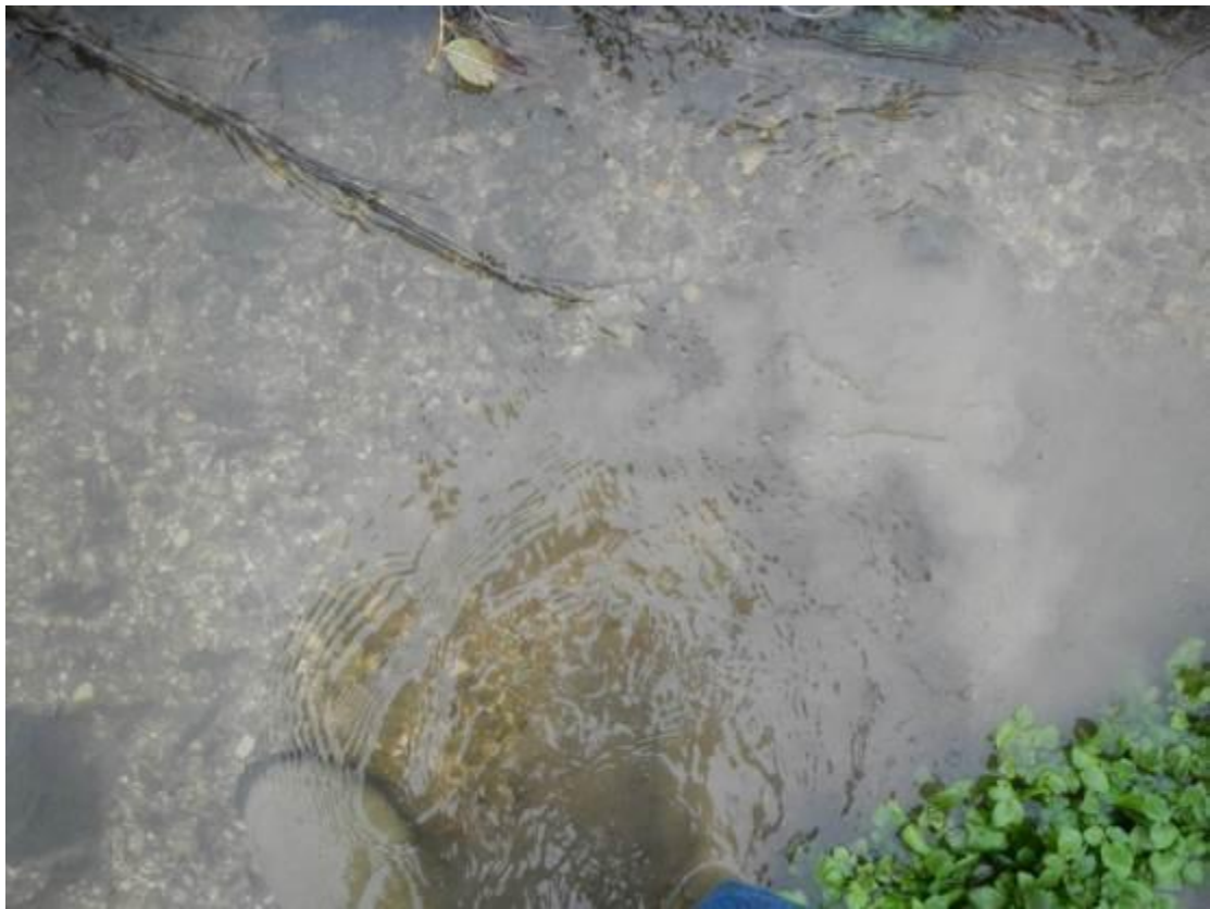
Figure 6. Agitating the bed liberates a volume of fine sediment.
