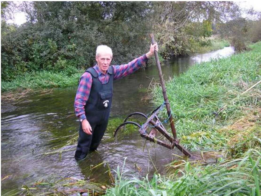
The "Ripper". A simple winch operated grapnel designed to grub out the roots of unwanted emergent plants.
