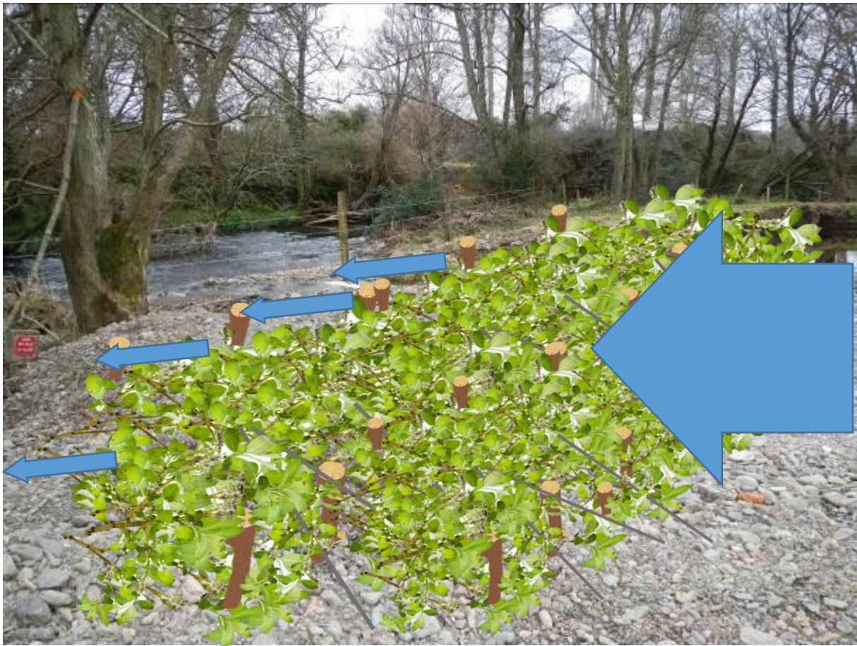
Figure 39. Slowing the transition of water across the bend and restricting its egress at the far side would greatly reduce the flow energy across the bend, reducing erosion and causing any bed material to be deposited there, turning it from an area of scour to an area of deposition. This would also encourage flows to follow the original channel course as the path of least resistance.
