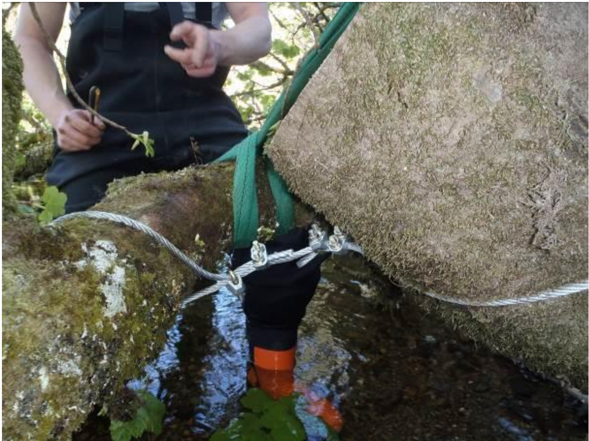
Figure 32. A basic tree kicker cable setup using 4000kg braking strain cable and two sets of cable clamps. The webbing strap in the background is used to pull the kicker close to the stump but is removed once the cable is fully fixed in place.
