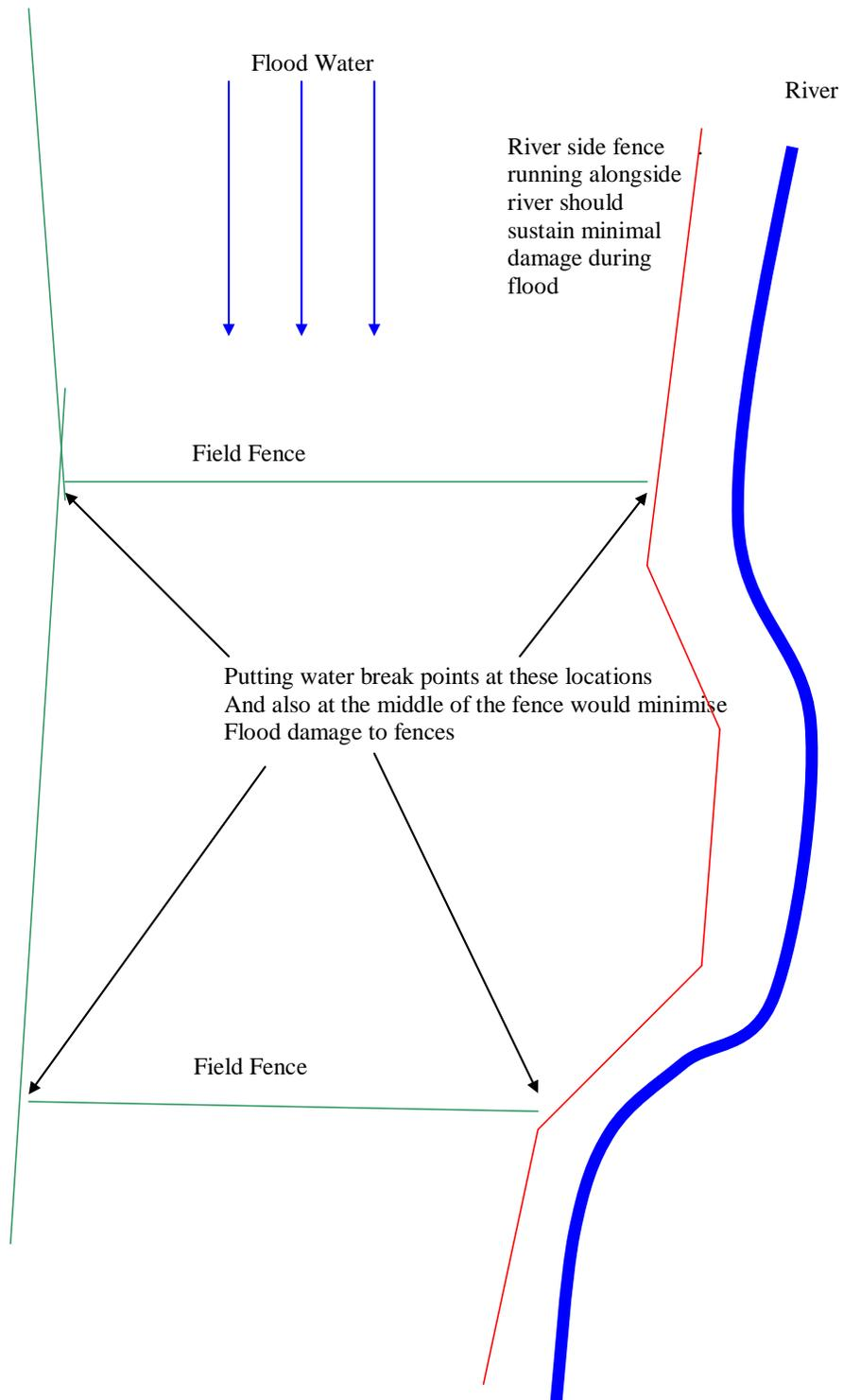
**Details for setting up water break points to separate one fence into two**
