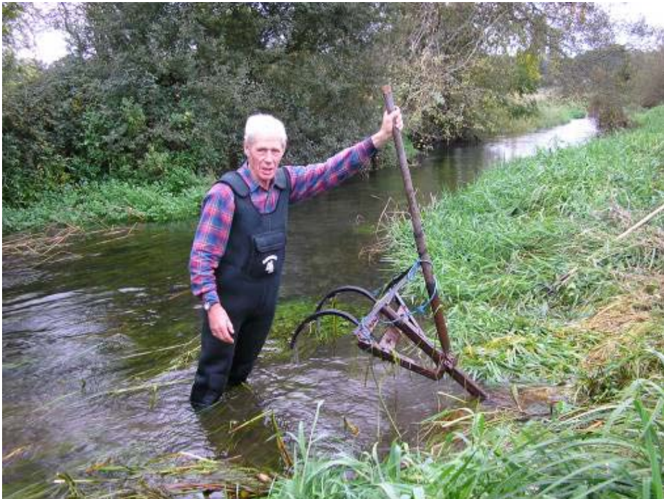
Anthony Mitchell with his winch driven "ripper" designed to remove pipe reeds from the Dorset Allen
