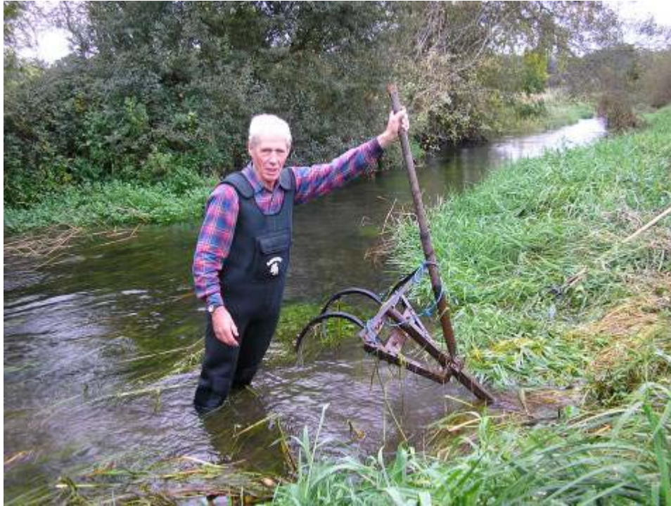
"The ripper" a simple plough designed to be used with a bank-side winch to grub out undesirable plants.
