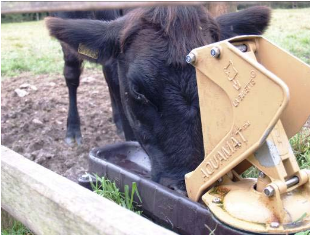
Pasture pump in use next to the River Test. No access for cattle to the river required
