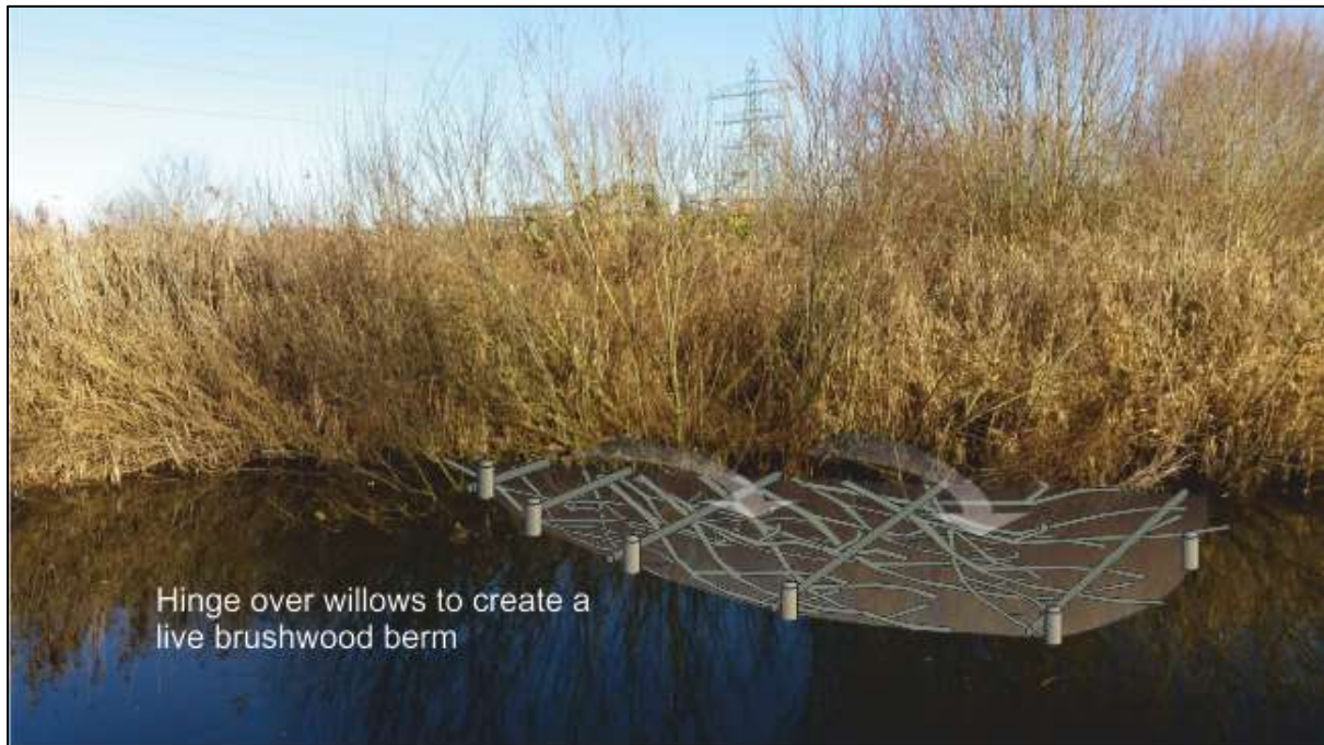
Figure 6: An illustration showing how clusters of branches could be hinged and secured to create a living brushwood berm
