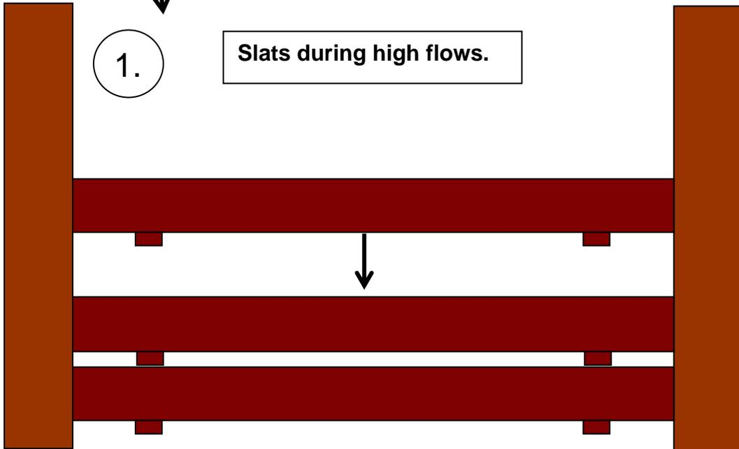
Construction of barrier. Ensure allowance is made for swelling of wood.
