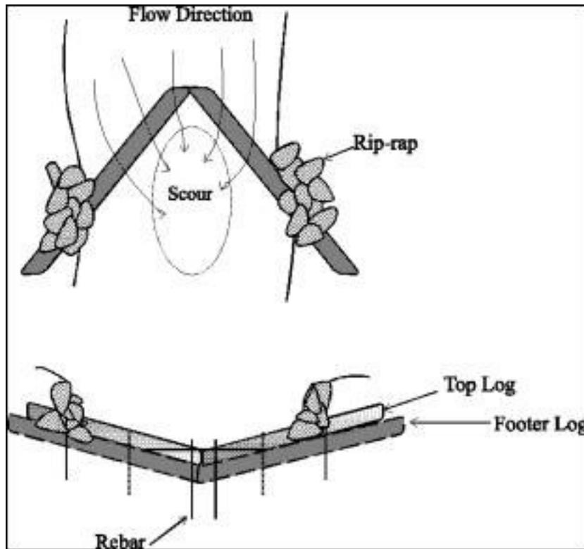
Figure 2. Upstream facing log V-weirs are a simple and cost effective way of increasing habitat, particularly for older trout.
