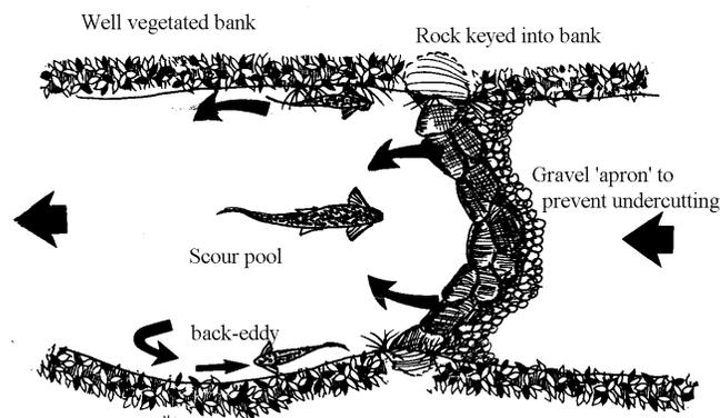
In small streams deep water adult trout habitat can readily be created by building upstream - curved weirs which concentrate flows in the centre of the channel. Cover logs along edges improve holding capacity.
