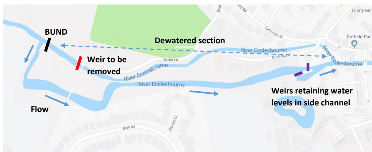
Figure 2 Position of bund for stages 1, 2 and 3 of the works, showing diversion of flow into side channel and de-watered section.
