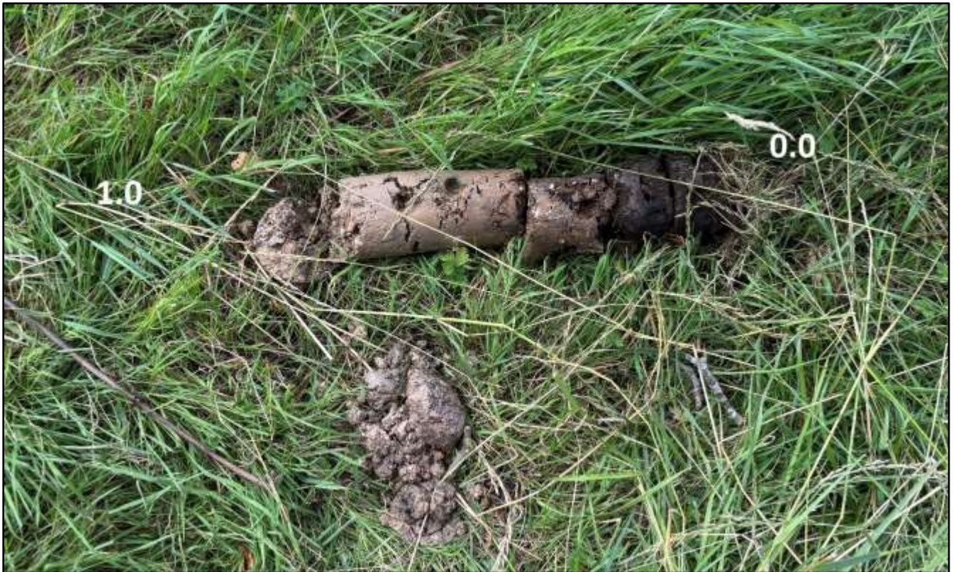
Fig 11 - core from BH6 (poor recovery)
