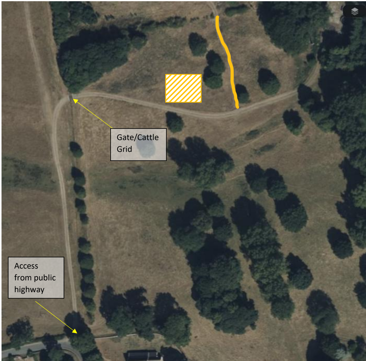
Figure 3 Site compound location (hatched area) and access route to spoil spreading area (orange line) from existing track.
